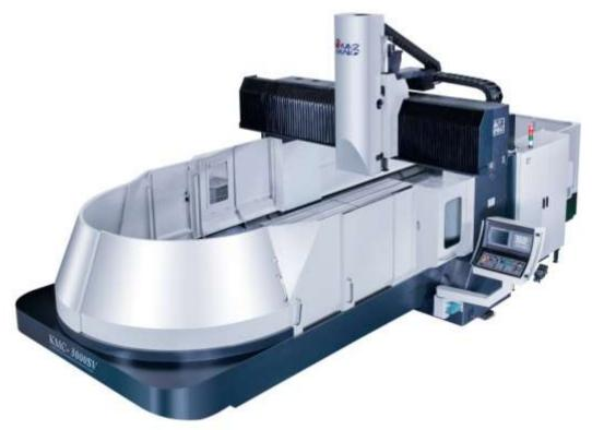
The Kao-Ming KMC-3000SVH 'C' 2.1 DBC 5 Face Machining Centre with High Torque has been installed for the machining of large steel components and structures with a capacity of (X) 3230mm x (Y) 1950mm x(Z) 775mm
