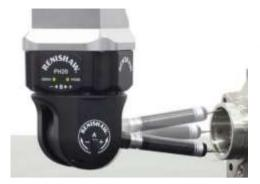
Quality is foremost in PRV Engineering's manufacturing philosophy, so, as well as installing the latest state of the art inspection probing systems on our machining centres, we have also Constructed a Temperature Controlled Inspection Department Housing a Renisahaw PH20, 5 Axis Touch Probe CNC Coordinate Measuring Machine utilising the latest MODUS software for programming and control along with a host of conventional inspection and testing equipment.
